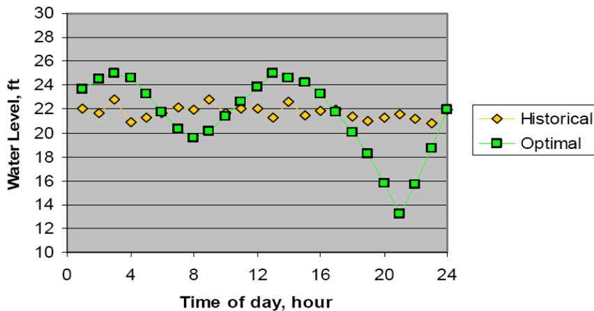
Figure 4: Reservoir water level is allowed to vary more in the optimized system as a consequence of less frequent pumping. Operators can be confident that the reserve will be sufficient to meet demand because the system accurately predicts future consumption and schedules accordingly.
