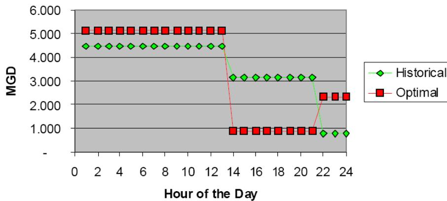
Figure 3: In the optimized system (in red) well production is minimized during on-peak hours in the afternoon and evening.
