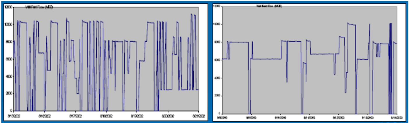
Figure 2: In the optimized system (on the right) pumps are used less often.
